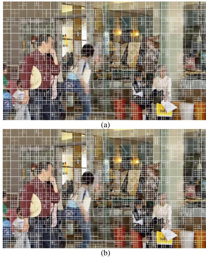
**Figure 3.5.** Performance partitioning of first frame of BQMall for QP22. (a) HM. (b) *Node64* proposal
