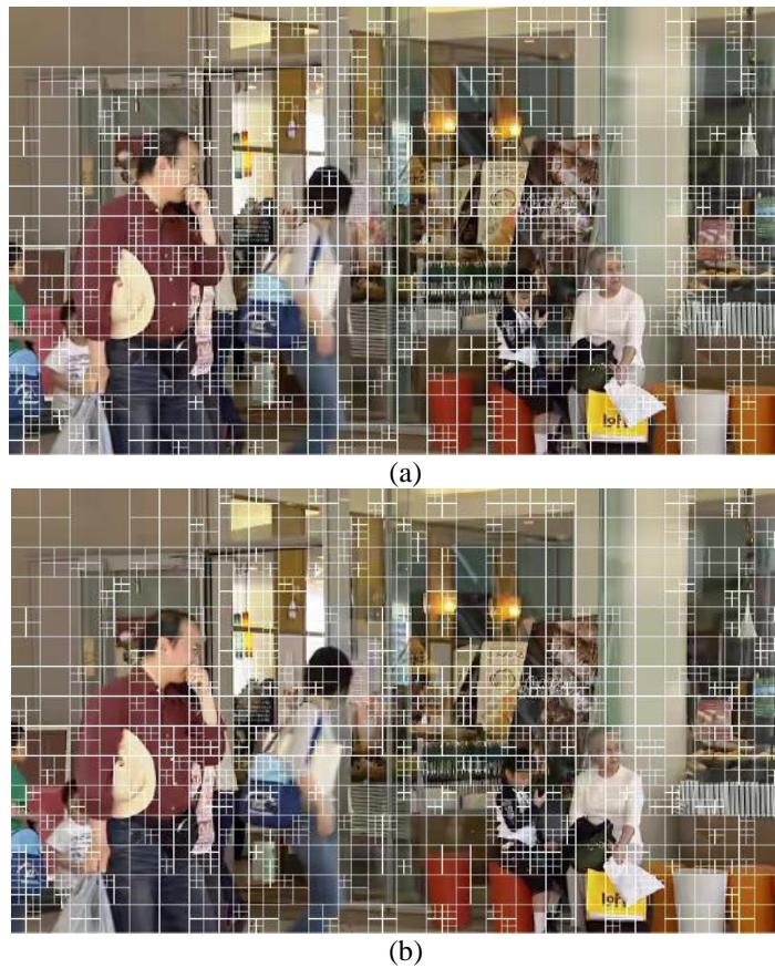
**Figure 3.6.** Performance partitioning of first frame of BQMall sequence for QP37. (a) HM. (b) *Node64* proposal
