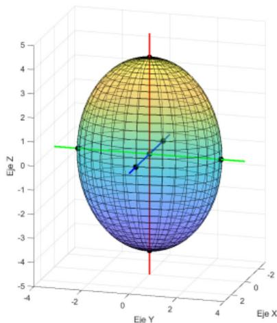
Figura: Elipsoide  $(x^2/4) + (y^2/9) + (z^2/16) = 1$
