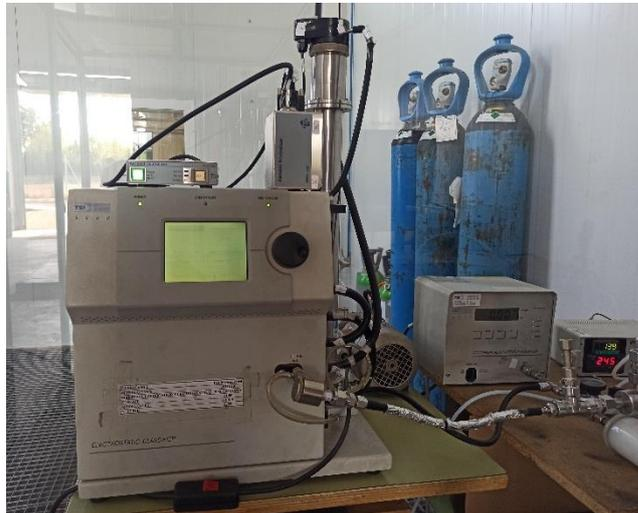
Figura 3.12 SMPS (*Scanning Mobility Particle Sizer*)
