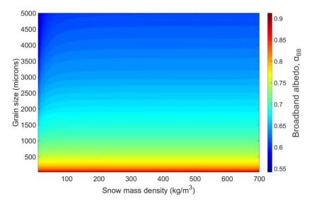
**Figure 3.** Broadband snow surface albedo  $\alpha_{BB}$  as a function of both snow grain radius and snow mass density calculated with the SNICAR model.  $\alpha_{BB}$  is largely insensitive to changes in snow density for snow densities greater than ~100 kg/m<sup>3</sup> and grain radii smaller than ~2000 µm.
