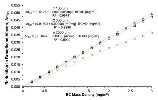
**Figure 5.** Reduction of snow surface albedo  $\Delta \alpha_{BB}$  as function of *BCMD* for three grain radii (i.e., 100, 500, and 2000 µm) and the resulting slopes *m* for *BCMD*  $\leq 3 \text{ mg/m}^2$  from a linear regression, where the error of *m* is the standard error value of the regression slope.
